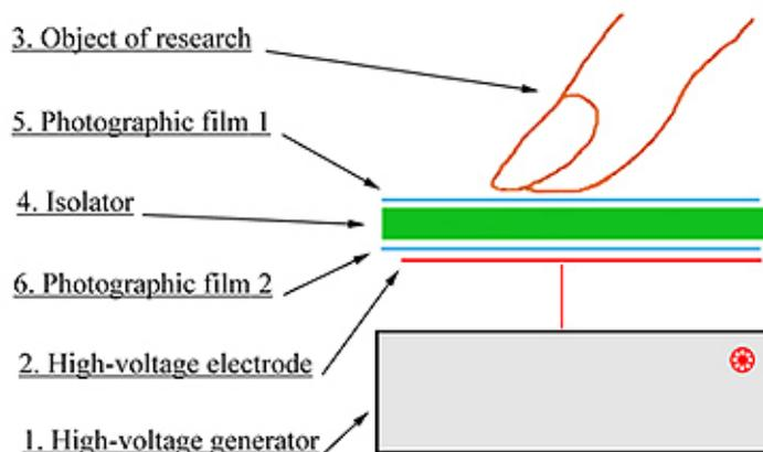
Figure 1. The scheme of a distant plasmagraphy
